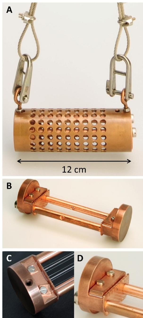
**Figure 2.** In-situ sampler. Full assembly (A), interior unit (B), holding fixture for hollow fibers (C) and glass fibers (D).
