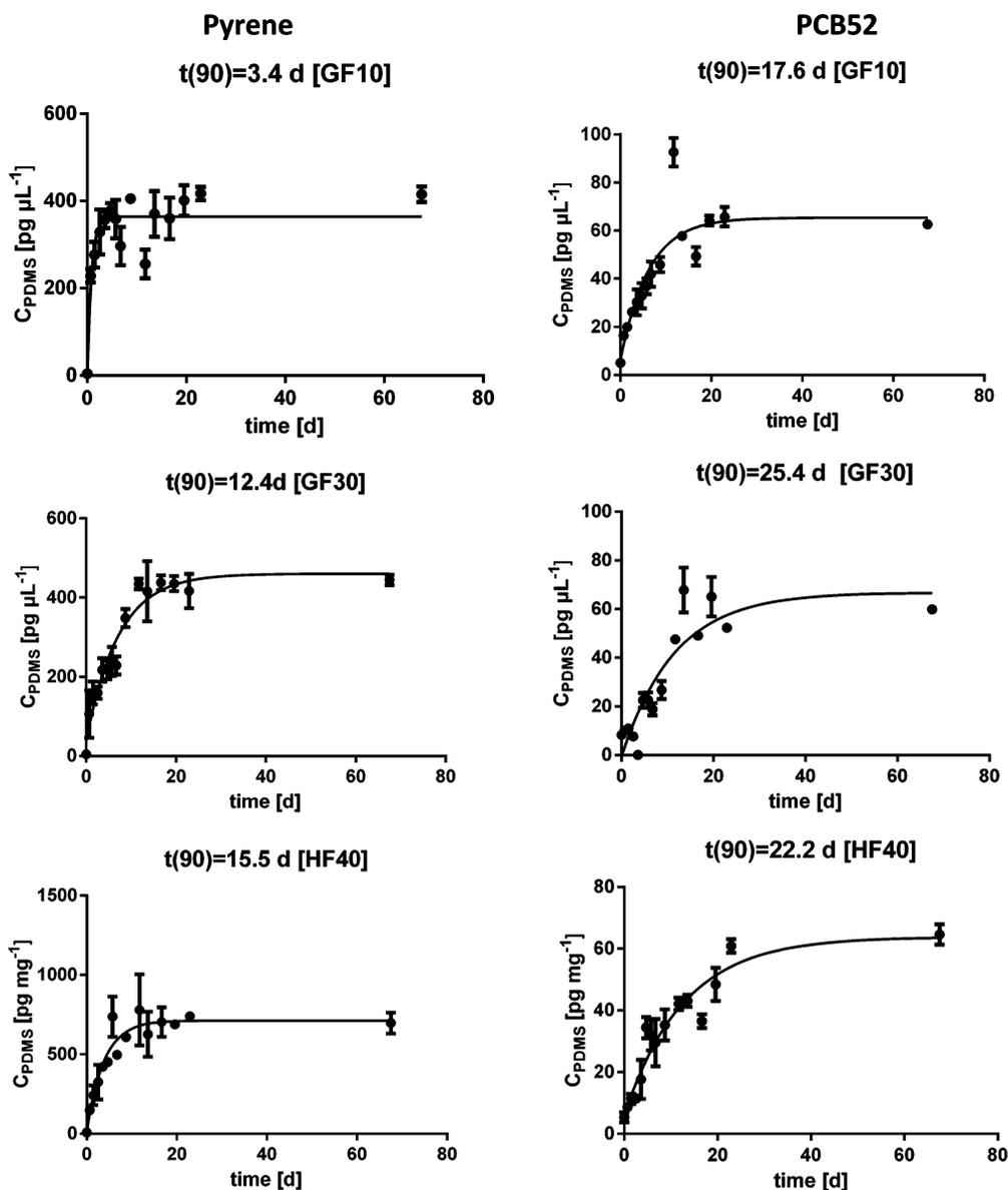
**Figure 3.** Example curves: uptake of contaminants into PDMS fibers with 10 and 30  $\mu\text{m}$  PDMS coating as well as hollow fibers with 40  $\mu\text{m}$  PDMS walls;  $t(90)$  values are given based on the upper confidence limits of model parameter estimation (mean values and standard deviation); drawn lines present first-order model fit.
