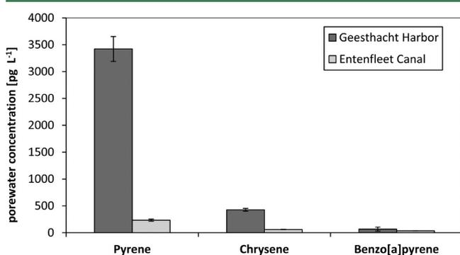
**Figure 5.** In-situ measurement of PAHs at a contaminated site (River Elbe near Geesthacht, Schleuseninsel Harbor;  $T = 20 \text{ }^{\circ}\text{C}$ ) and a pristine canal (Entenfleet during winter,  $T = 4 \text{ }^{\circ}\text{C}$ ); experiments were performed with GF10 fibers and  $C_{free}$  was temperature corrected for winter.
