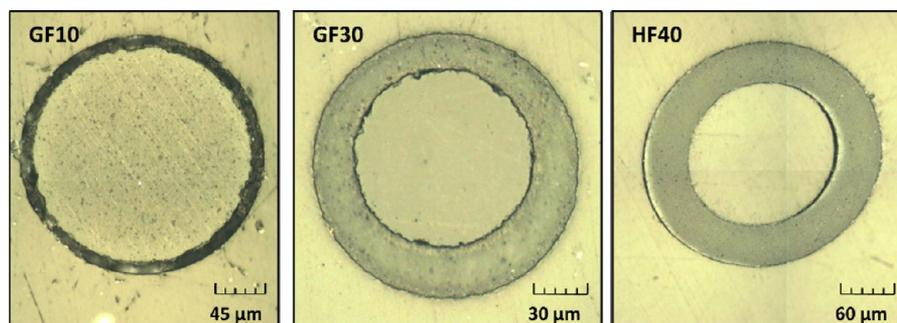
**Figure 1.** Photographic images of the fiber coatings measured with laser scanning confocal technology (OLS3000 LEXT Microscope); submicrometer imaging with 0.12  $\mu\text{m}$  resolution.
