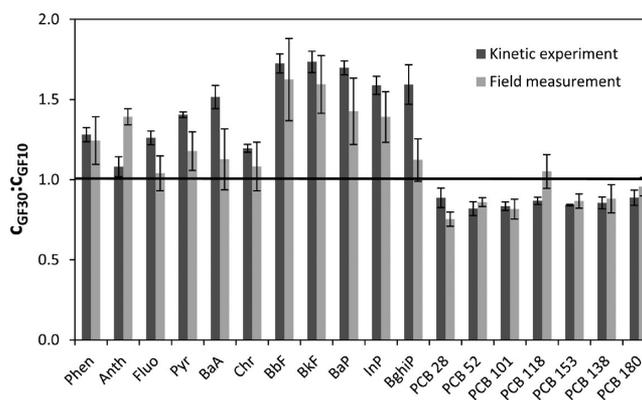
**Figure 6.** Concentration ratios between two coexposed PDMS coatings ( $C_{GF30}:C_{GF10}$ ) from in situ deployment in River Elbe sediment and the equilibrium phase of the kinetic experiment. The good agreement of in situ and laboratory ratios supports fulfillment of the equilibrium criterion for the in situ sampling.
